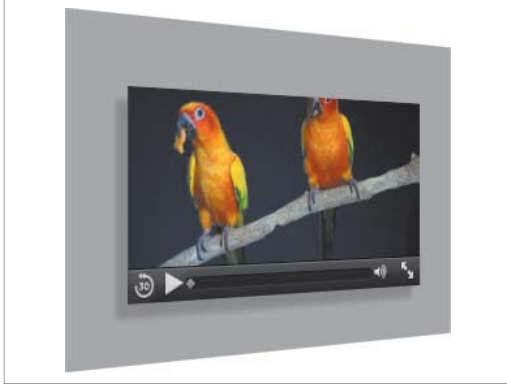
FIGURE 7.14 The video and background div are rotated at a 40-degree angle around the Y axis in Safari 5.1.
