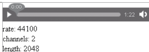
FIGURE 11.1 The audio file's sample rate, channels, and buffer length are displayed onscreen in Firefox 6.
