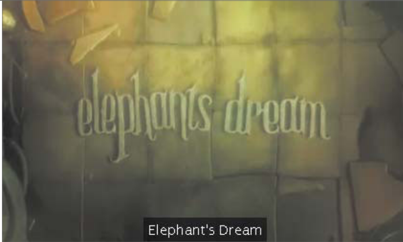
FIGURE 8.1 How a subtitle cue might appear on a video with no cue settings specified.
